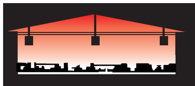
● BLOWN AIR SYSTEMS WASTE ENERGY IN THE ROOF SPACE AND HEAT YOUR WORKING AREA LAST.
